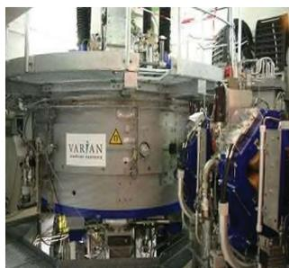
Magnete SC di Varian (90 Ton, Isochronous Cyclotron)
